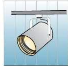
Track Lighting (Incandescent)
